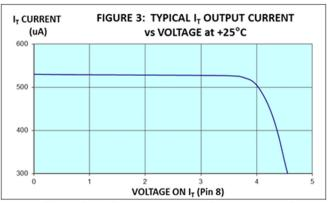
Keep Pin 8 voltage in 0 to +3V range for proper readings.
